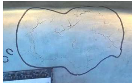
Thermal fatigue crack, SPF matrix
