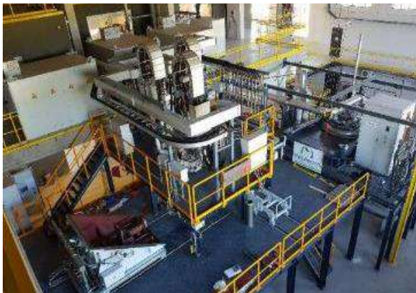
PAM-CHR - Plasma Arc Melter, Cold Hearth Refiner
