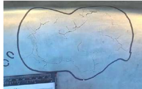
Thermal fatigue crack, SPF matrix
