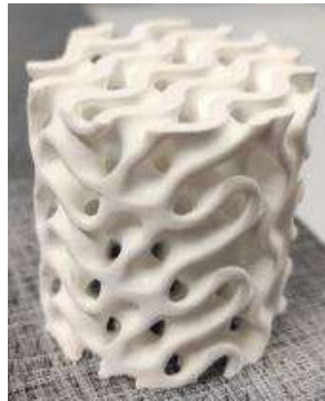
Figure 1. 3Y – TZP Gyroid Ceramic Monoliths produced by Digital Light Processing
